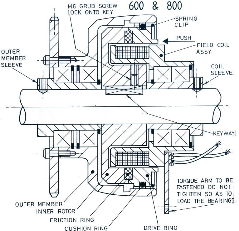
THE CLUTCH MAY NOT "PULL IN" WHEN THE COIL IS FIRST ENERGISED. WITH THE INPUT DRIVE STATIC AND THE FULL 24 VOLT DC SWITCHED ON, THE DRIVE RING SHOULD BE EASED TOWARD THE INNER ROTOR UNTIL IT PULLS IN.
