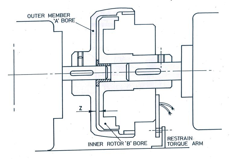
TO ASSIST THE ALIGNMENT OF THE SHAFTS BEING COUPLED WITH A BM TYPE CLUTCH USE A PILOT BEARING IN THE END OF THE INNER ROTOR.
