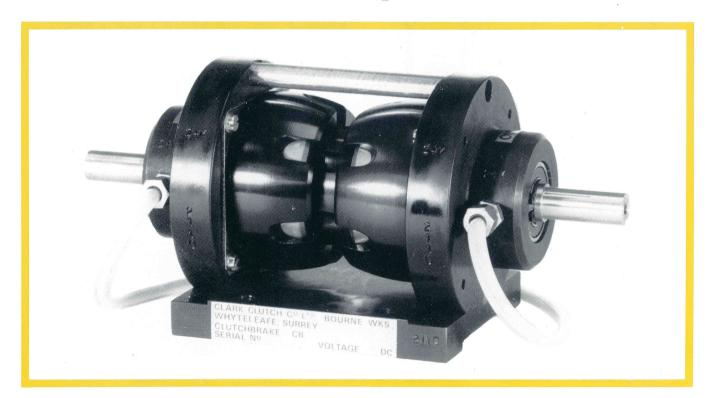
The Clark Composite Clutchbrake unit is a combination assembly of the well proven Clark model 250 Clutch and Brake. Integral input and output shafts running in substantial sealed bearings reduce fitting to the ultimate in simplicity and low cost. The unit requires no maintenance and is entirely self-adjusting.
